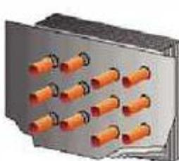
Due to the thermal expansion of the copper pipes, all metal sheets are equipped with an aluminium plate with collars. This plate supports the tube and therefore the pipes must not come into contact with the metal sheets. With this solution, the vibrations and thermal expansion are absorbed by the aluminium sheet. Leaks caused by friction cannot occur. The rigidity of the coil is sustained effectively.
